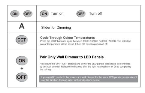
To use both the remote and wall dimmers for the same LED panels, first pair the remote with the LED panels. Then, pair the wall dimmers with the remote by holding down for 5s the below combination of buttons.
